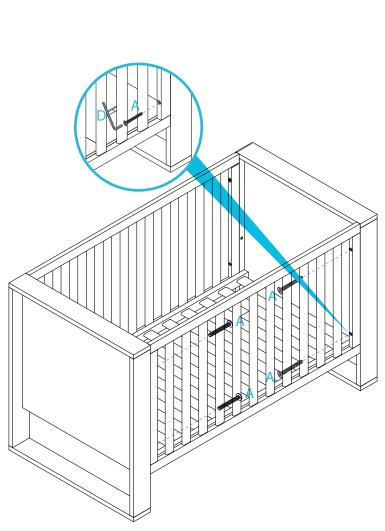
Turn the cot over so the bottom of cot is at the top.Attach the cot base to the required level(newborn or Toddler) using 4 x screws(B) as shown and tighten with allen key.Pictured is the lower toddler base.The higher newborn level is closer to the top rail of the cot.
