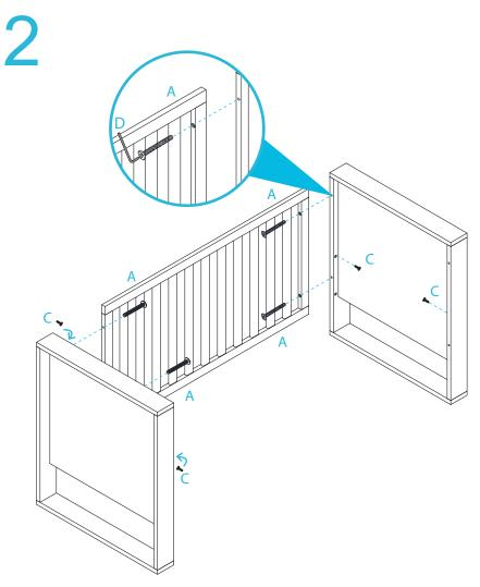
Insert 4x screws (C) in the holes as shown. Tighten with the Allen key (D)
